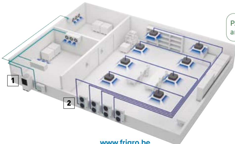
1 Condensing units – iCORE and iCOOL ranges for refrigerated room.
